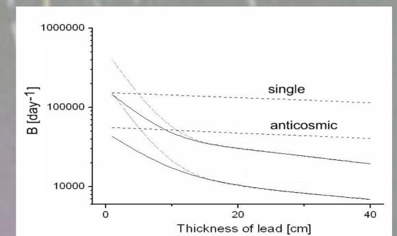
Figure 4. Total background counts (0-3000 keV) due to hard (broken line), soft (dotted line) and nucleonic (solid line) components.
