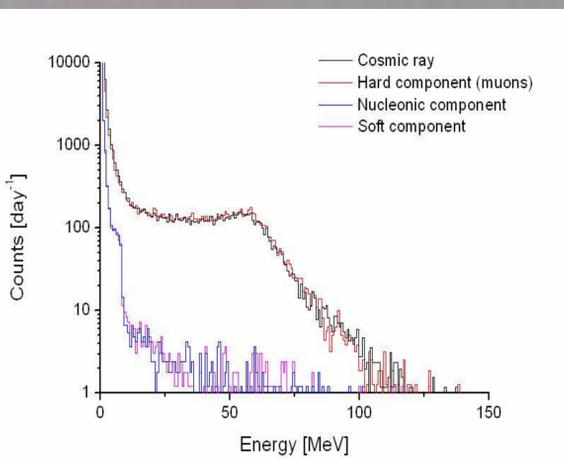
Figure 3. High-energy spectra of different components of cosmic rays at sea-level with antic cosmic shielding predicted by Monte Carlo simulation.
