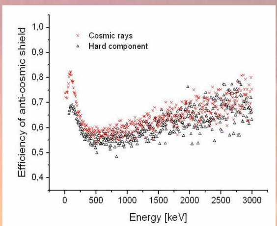
Figure 5. Efficiency of the antic cosmic shielding as a function of the energy for hard component and all cosmic rays.
