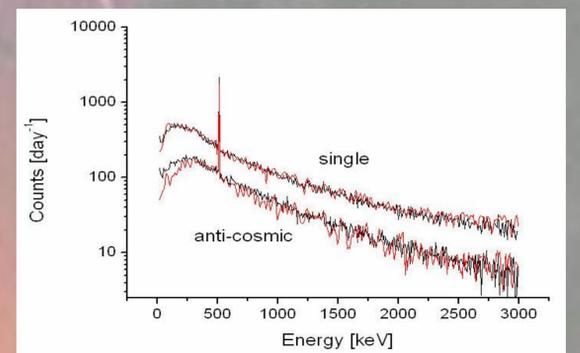
Figure 6. Low-energy spectra of hard component (red line) and all of cosmic rays (black line) at 10 m w.e. underground for a single and antic cosmic spectrometer.
