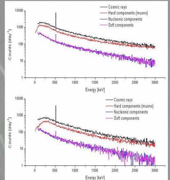
Figure 2. Low-energy spectra of different components of cosmic rays at sea-level in a single Ge spectrometer (top), and with antic cosmic shielding (bottom) as predicted by Monte Carlo simulation.
